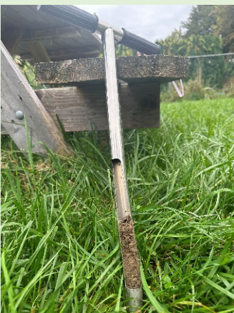
Method 1: Use a soil probe to take a soil sample to a depth of 6"
