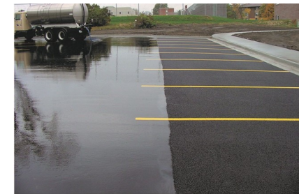
A visual demonstration of porous vs. impermeable asphalt.
