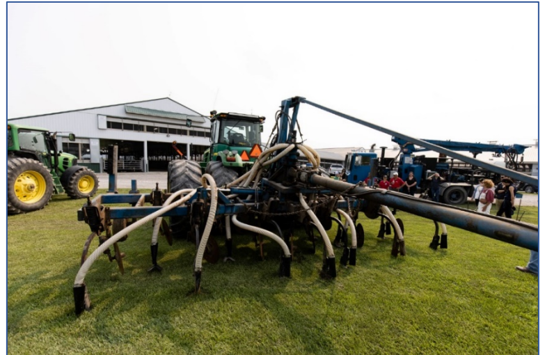
Manure injection (using a toolbar like the one pictured above) allows farmers to protect manure nutrients from runoff and allows for minimal soil disturbance. (photo: Partners for Healthy Watersheds)
